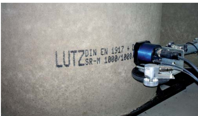
Marking of precast concrete pipes
