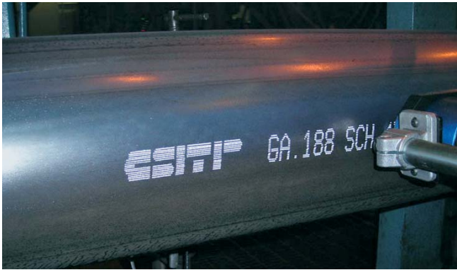
Marking of steel pipes
