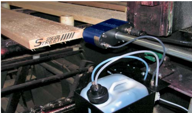
Marking on rough sawn timber boards
