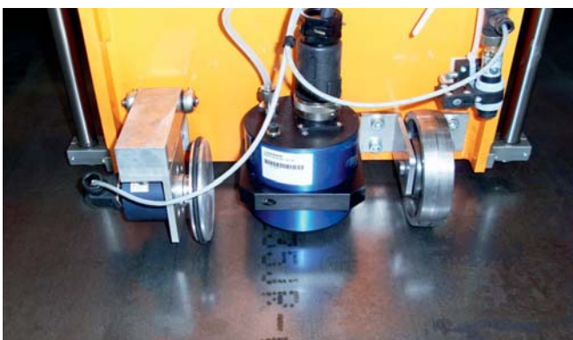
Steel sheet marking with etching ink
