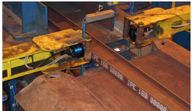
Marking of H-beams
