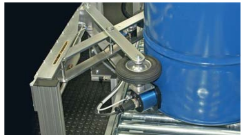
Barrel turning device
