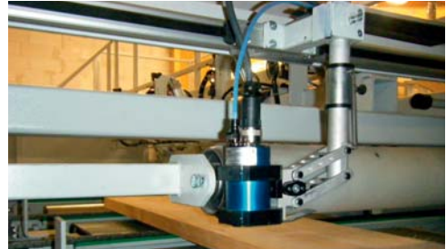
Vertical distance levelling device
