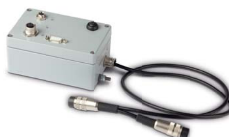
Flyback Compensating Device
