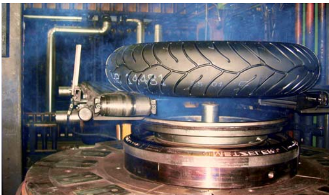
Tire marking with Naphtha-ink
