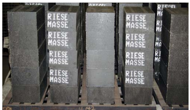
Refractory stone marking with high-temperature ink
