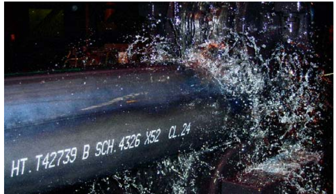
Steel tube marking with pigmented MEK ink
